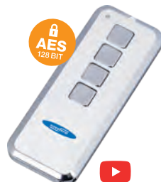
Mini-Novotron 524 Design* 4-Kanal, 433 MHz, KeeLoq-Wechselcode
